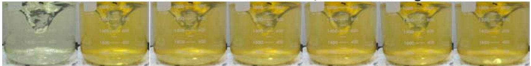
Ferrous Sulfate Fenton Reaction, From Left to Right: 0-30min
