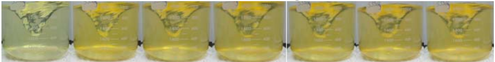
Ammonium Ferrous Sulfate Fenton Reaction, From Left to Right: 0-30min
