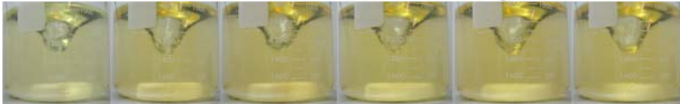
Ferric Chloride Fenton Reaction, From Left to Right: 0-30min
